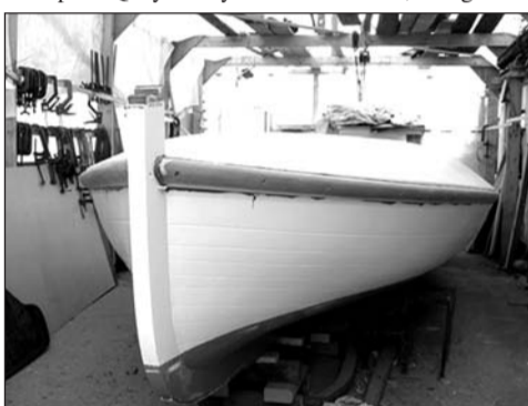
The restored "Terror" nearing completion
